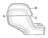
To access the upper storage area, press the upper button (B) and lift up. To access the lower storage area, press the lower button (C) and lift up. The top of the console can be folded forward for increased storage area. Lift up on handle on the rear of the console (A) and pull forward.
